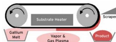
Planned nanowire production reactor (kgs/day) that has rapid reaction capability.
