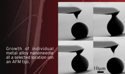
Growth of individual metal alloy nanoneedle at a selected location (on an AFM tip).
