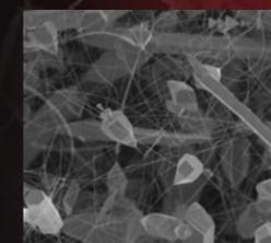
Handles on GaN nanowires. Tapered GaN crystals that were grown onto existing GaN nanowires.
