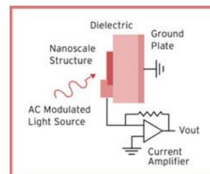
UofL's femtosecond spectroscopy method for single nanowires.
