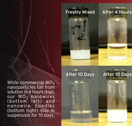
While commercial WO<sub>3</sub> nanoparticles fall from solution in 4 hours (top), our WO<sub>3</sub> nanowires (bottom left) and nanowire bundles (bottom right) stay in suspension for 10 days.
