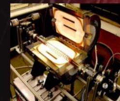
An experimental reactor for evaluating principles for the bulk production of nanowires.
