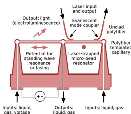
A multifunctional microsystem device concept configured around the ability to make suspended polymer fibers in one step.
