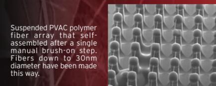
Suspended PVAC polymer fiber array that self-assembled after a single brush-on step. Fibers down to 30nm diameter have been made this way.
