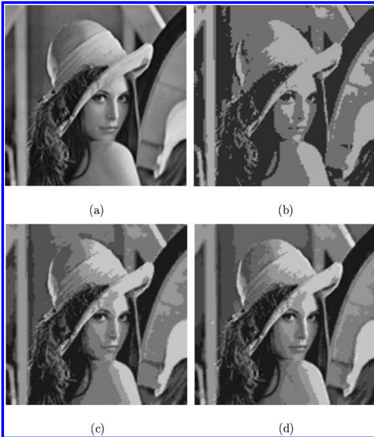
Figure 6: Image segmentation worked with a 128 \times 128 Lena image using the SCLM method. (a) Original image. (b) Image segmented with three layers. (c) Image segmented with six layers. (d) Image segmented with nine layers.
